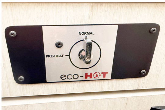
Eco-hot valve in Normal Position (Located passenger side on the sink.) -Typical View
