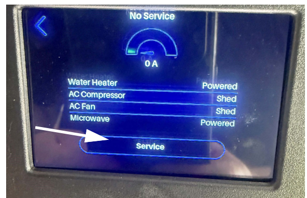
Power Control System screen. Select the Service button to select the shore power service. -Typical View
