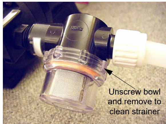
Water Pump Strainer -Typical View
