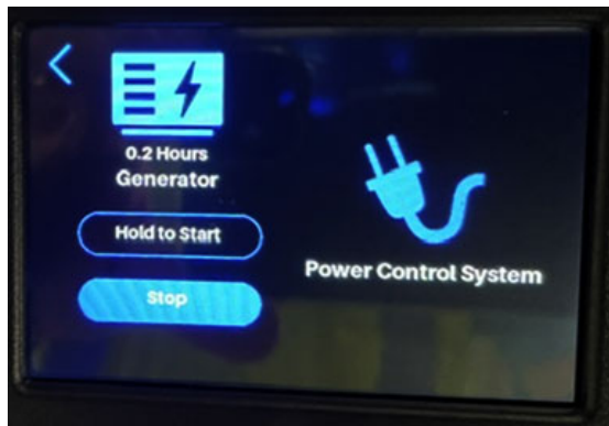
Select the Power Icon on the main menu to access the Generator start/stop screen. -Typical View
