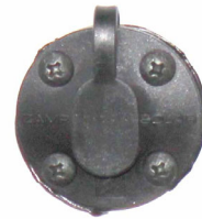
Exterior Solar Port (Located on the driver's side exterior of motorhome). -Typical View
